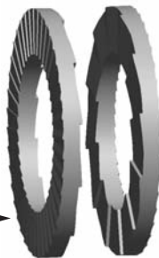
Nord-Lok™ Washers – Coarser serrations must face inward and lock together
